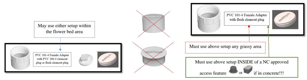
Leave the cleanout fittings **UNGLUED** at time of W&S installation (to be lowered and glued in place after finish grade).
